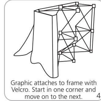
Graphic attaches to frame with Velcro. Start in one corner and move on to the next. 4
