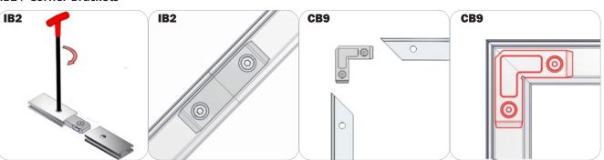
Press the hex bolt head in with your thumb and slide the extrusion and connector together so that the hex bolt head sits into the lock hole. Repeat with the second extrusion to the free end of the connector. Lock the extrusions together by turning carefully with the allen key tool. Be sure to lock securely, but do not overtighten.
