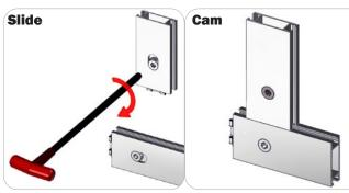
A cam lock equipped extrusion can lock to any cam lock channel. With the cam lock unlocked, set the teeth of the cam lock into the desired position on the cam lock channel. Using your allen key tool, carefully turn the lock clockwise to lock in place. Be sure to lock securely, but do not overtighten.
