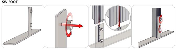
An SW-FOOT assembly consists of two thumb screws, an LN100, and SW-FOOT baseplate. Start by loosening the thumb screws (it is best not to completely remove the screws). Slide the extrusion onto the LN100 by utilizing its back cam channel. When the extrusion rests on baseplate or ground (depending on application), tighten the thumb screws to lock in place. Do not overtighten.
